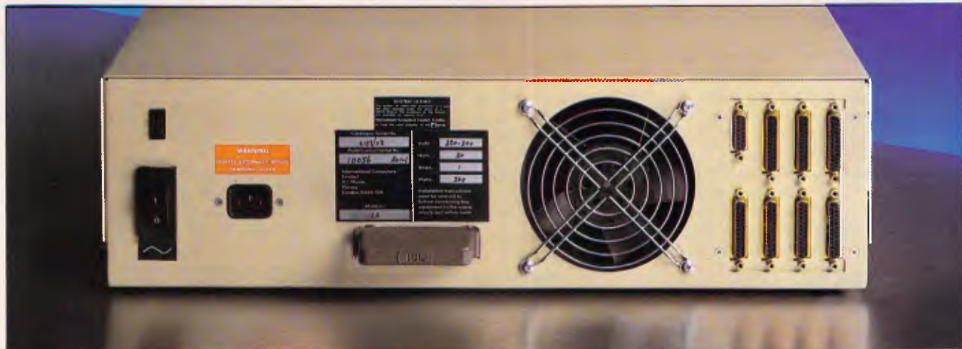
An interesting rear view: up to four workstations can be connected
